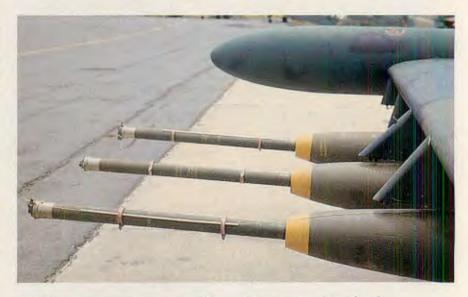
ABOVE: Three-foot fuse extenders on 500-pound bombs ensure detonation above ground level for maximum shrapnel effect. BELOW: Twin M60s in each door of a Huey make it a "gunship." Photos: Dana Drenkowski
